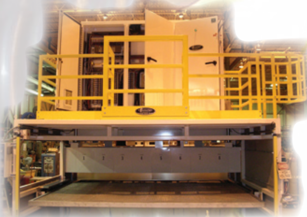
Mezzanine mounted control panel for thermoforming ovens
